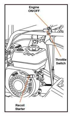
To stop the engine in an emergency, simply turn the engine switch to the OFF position. Under normal conditions, use the following procedure.
