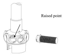
**3.** Check the air release hose are fixed well on the body of lateral holder, and another end of the air release hose must be out of the sand. DO NOT embedding the air release hose in the sand.
