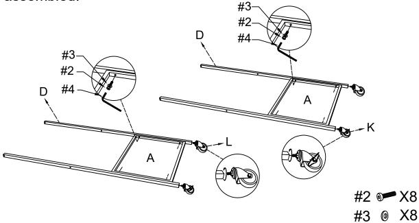
**Step 2.** Attach short side panels (part B) to long side panels (part A) of assembled parts (part A,D,L&K) using long bolts (part #2), washers (part #3) and allen key (part #4).
