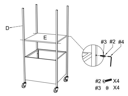
**Step 6.** Attach top frame (part F) to long posts (part D) of assembled parts (part A,B,C,D,E,L&K) using long bolts (part #2), washers (part #3) and allen key (part #4).
