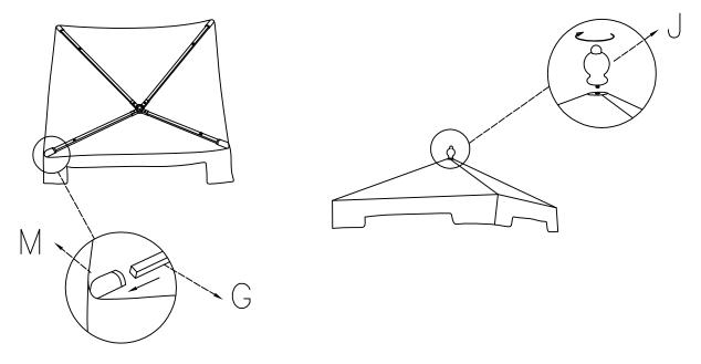
**Step 10.** Attach assembled parts (part G,H,J&M) to connectors (part I) of assembled parts (part A,B,C,D,E,F,I,L&K) using short bolts (part #1), washers (part #3) and allen key (part #4).
