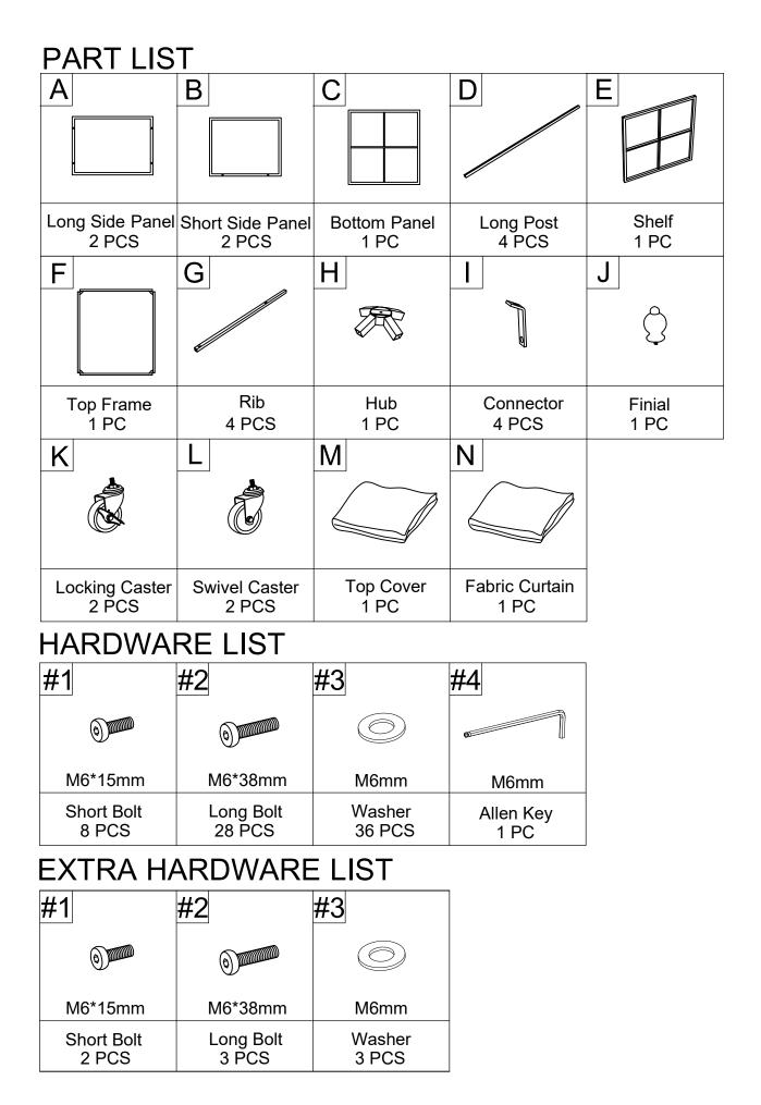
Step 1. Attach long side panels (part A) to long posts (part D) using the long bolts (part #2), washers (part #3) and allen key (part #4).Attach swivel casters (part L) and locking casters (part K) to long posts (part D).
