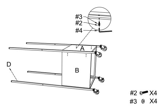
Step 4. Attach bottom panel (part C) to short side panels (part B) of assembled parts (part A,B,D,L&K) using long bolts (part #2), washers (part #3) and allen key (part #4).
