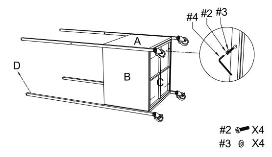
**Step 5.** Attach shelf (part E) to long posts (part D) of assembled parts (part A,B,C,D,L&K) using long bolts (part #2), washers (part #3) and allen key (part #4).
