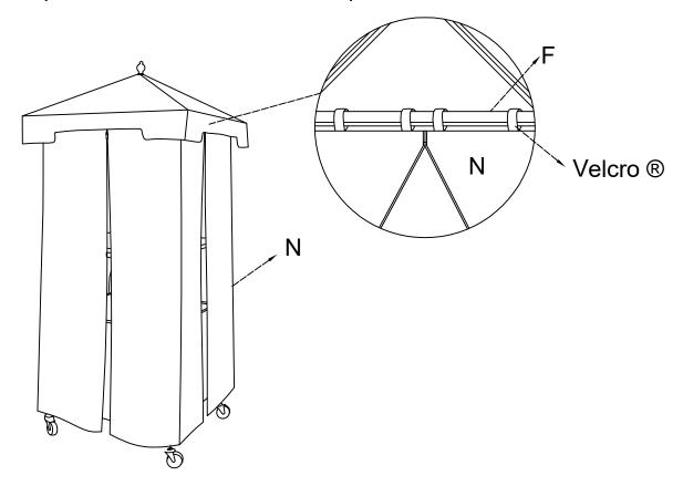
**Step 12.** NOTE: Curtains (part N) can be held open by using the Velcro ® straps to secure them to long posts (part D) of the completed unit as shown below.
