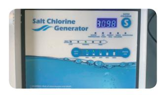
**Step 11.** After a couple of minutes, the controller display will show a salt value of between 2700 and 3400 and the "Power" and "Generating" LEDs should be light on.
