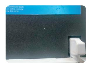
**Step 8.** Plug the power cord into the lower corner of the controller.
