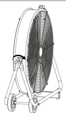
Adjust the locking knobs to secure the drum in desired position, and tight it by turning the locking knobs clockwise.
