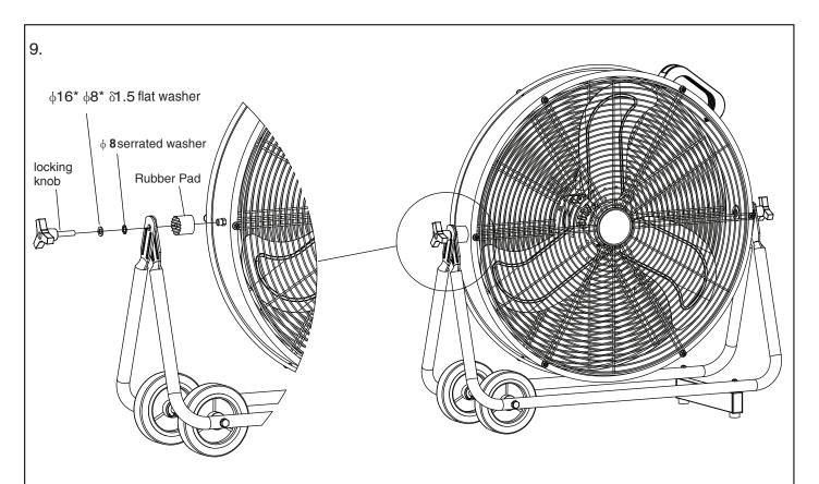
Assemble the base bracket with two side of drum body by fastening the locking knobs, flat washers, serrated washers and rubber pads.
