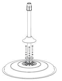
3. Slide the height adapter into the upper standing pole. Then put the upper standing pole into lower standing pole and fasten the height adapter for your desired height of fan.
