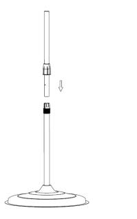
2. Loosen the height adapter on the lower standing pole. Saving it for Step 3.
