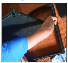
**Step 2:** Attach the back of the chair onto the backside of the seat portion of the chair using a M6  $\times$  15 bolt.
