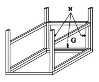
**STEP 6:**Connect the part :from step **S** and table Side frame **O** with bolt N with alien key
