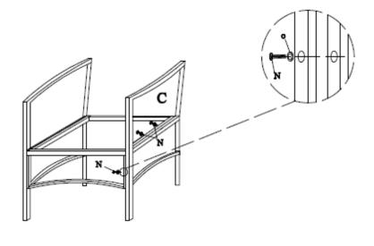
**STEP 2:**Connect the parts from step 1 to the right frame **C** with bolt **N** and secure it with an allen wrench.
