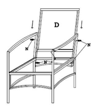
**STEP 3:**Connect the parts from step 2 and back frame **D** with bolt **N** with an allen key.
