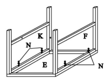
**STEP 5:**Connect Table frame **F, K** & table Tabletop frame **B** with bolt **N** with allen key
