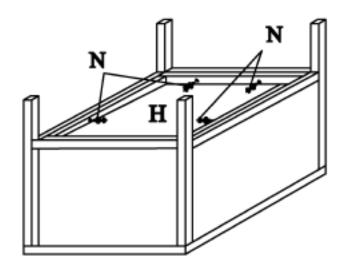
**STEP 7:**Connect the part from step 6 and table under frame **H** with bolt **N** with a1len key
