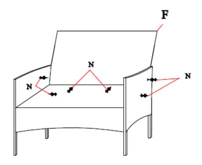
STEP 7: Connect the part from step 6 and bench back frame F with bolt N with Allen key.
