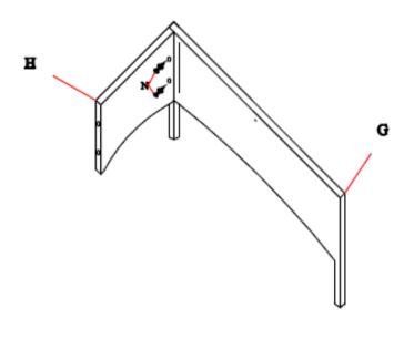
STEP 9: Connect Table leg frame G & table side frame H with bolt N with the Allen key.
