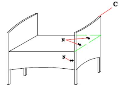
STEP 5: Connect left frame B & bench seat frame E with bolt N with Allen key.
