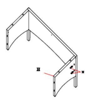
STEP 10: Connect the part from step 9 and the table side frame H with bolt N and secure with Allen key.
