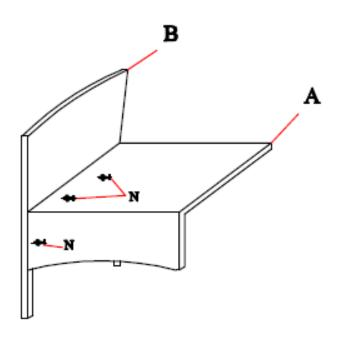
STEP 1: Connect left frame (B) and seat frame (A) with bolt (N) and secure wit the Allen key.
