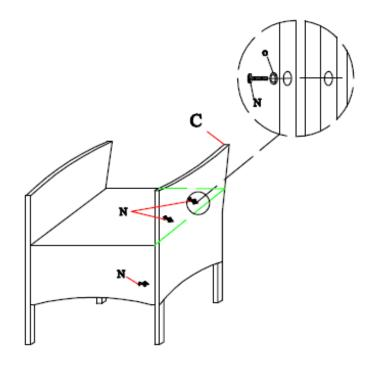
STEP 2: Connect the parts from step 1 to the right frame (C) with bolt (N) and secure it with an Allen wrench.
