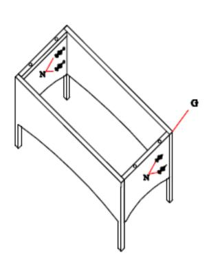
STEP 11: Connect the part from step 10 and Table leg frame G with bolt N secure with Allen key.
