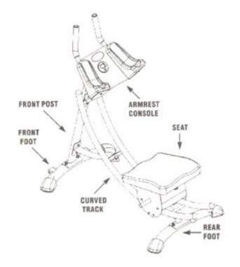
**Step 1:** Attach the rear foot to the rear of the curved track. Remove the 2 bolts which have been pre-attached to the rear foot, then re-attach the bolts to connect the foot to the track. Finger tighten the bolts only. DO NOT tighten the bolts with a tool until the unit is fully assembled.
