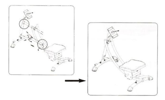
**Step 4:** Attach the armrest console to the top of the front post using the 4 pre-attached Allen head screws. Tighten all bolts and screws using the tools provided. Cover the bolts with black plastic caps provided.
