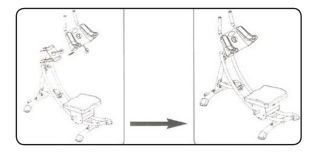
**Step 5:** Connect the counter wires in 2 locations as shown. Install the wire protection covers to cover the wire connections.
