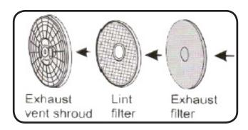
Separate each of the above parts and clean the individual pieces using a soft brush or vacuum cleaner. DO NOT damage the filters.
