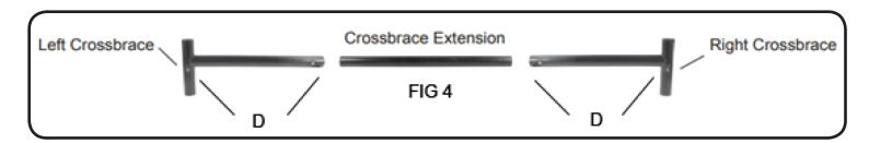
**STEP 3.** Insert the crossbrace into the crossbrace extension (Fig 4) and set the entire assembly on top of the upright legs. Center the crossbrace left to right and secure it with the allen head set screws (D). Secure the crossbrace to each upright leg with the included allen head set screws.
