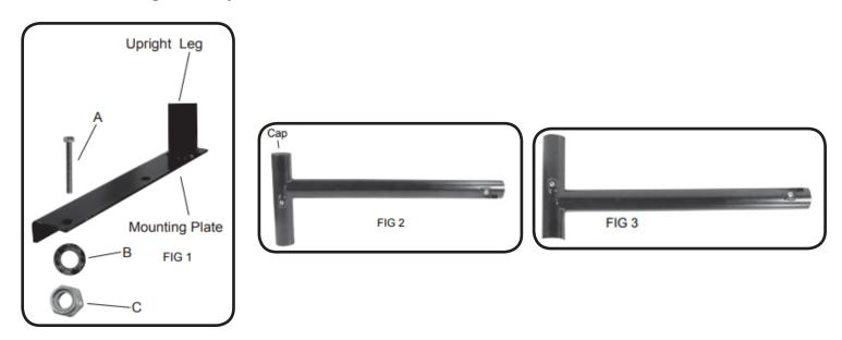
**STEP 2.** Set the rack to the high (FIG 2) or low (FIG 3) position, whichever is best for the cargo and the truck, by flipping the Crossbrace. For bowed canoes, the high position is recommended. If you choose to flip the Crossbrace, you will have to remove and replace the Caps.
