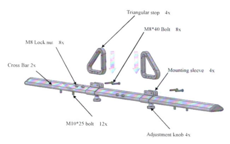
2. Tighten post A (1) and assemble cross bar with M10\*25 bolt (7), 10 spring washer (8), 10 washer (17) and M10 locking nut (16).
