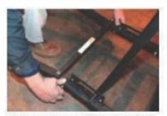
Remove two locking pins from the assembled base section.
