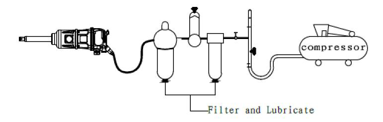
This Air Impact Wrench is made of wear-resistant and shockproof materials under strict quality control. Before each use, make sure to lubricate the tool with 3 - 5 drops of engine oil through the air inlet. Do not add oil with high viscosity. Re-connect air. Run impact wrench at low throttle without load for a few seconds to distribute the oil throughout tool.
