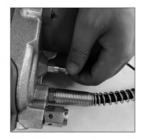
4. Unscrew the vent valve to empty the air in the oil reservoir casing(Note: a small amount of grease will be released).
