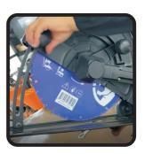
5. Attach the stationary knob and confirm it will allow you to adjust the depth.
