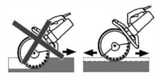
• Feed down the machine in line with the blade. Pressure from the side can damage the blade and is very dangerous.
