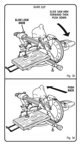
Release the switch trigger and allow the saw blade to stop rotating before raising the blade out of workpiece and removing the workpiece from miter table.
