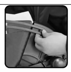
4. Connect the other side of the guide using a screw nut.
