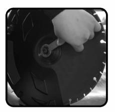
2. Secure the blade into the saw and tighten the bolt.
