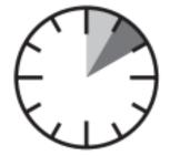
50% Rated Duty Cycle at 2.5 kVA output 5 seconds welding followed by 5 seconds of rest
