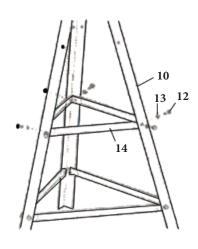
2. Tripod Assembly : Attach the pull rod (11) with the support pillar (10), using the plain washer M8 (13) and bolt M8x16 (12). Attach the short pull rod (14) with the support pillar (10) using the plain washer M8 (13) and bolt M8x16 (12).
