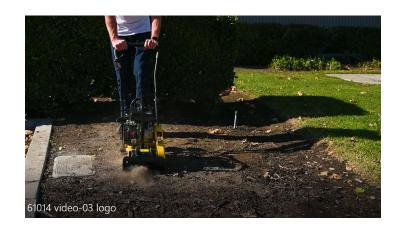
EFFICIENT COMPACTION OF COHESIVE SOIL, DEBRIS AND GRANULAR AGGREGATE MATERIALS UP TO 6.4"
