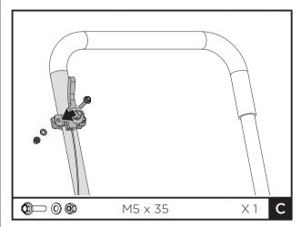
Unscrew bolt M5X35 from throttle control. Secure the throttle control onto the upper handle with a flat washer 5 and the bolt M5X35 that just were unscrewed.
