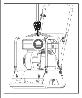
The unit must be transported in the upright position to prevent fuel from spilling. Do not lay machine on its side or top.
