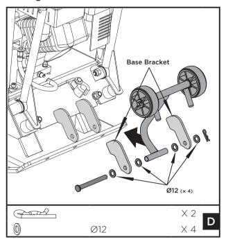
Align the holes on the wheel bracket shaft with the holes on the base bracket. Insert the 12x80 pin through the holes with one flat washer on each side of the base bracket plates. Then install the cotter pin. Using pliers bend and spread all the cotter pins prongs in opposite directions.
