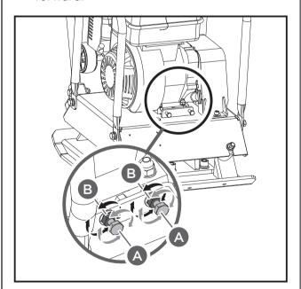
2. Loosen the jam nuts B, leaving enough space between the nut and bracket.
