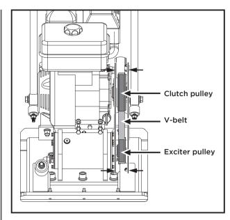
3. Push engine toward the back of the plate by turning the adjustment bolts A to remove any slack in V-belt(s).
