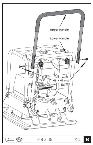
Mount the handle to the chassis with the button-headed bolt and knob-handle.
