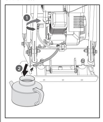
Running the engine with dirty oil can cause premature engine wear and failure. Changing oil regularly is extremely important. The flexible oil drain hose is equipped to drain oil into appropriate receptacle.
