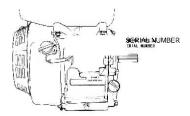
Record the engine serial number in the space below. You will need this serial number when ordering parts, and when making technical or warranty inquires.
