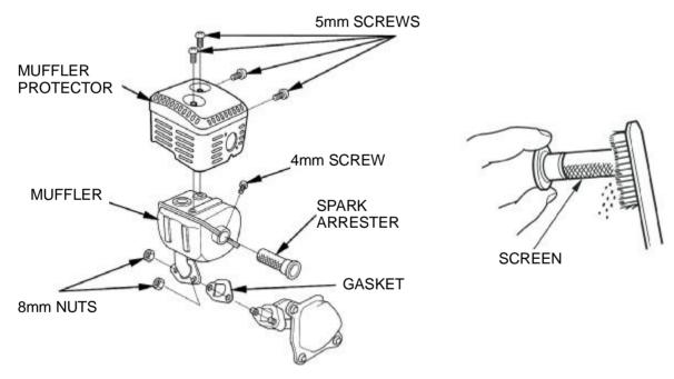
4. Use a brush to remove carbon deposits from the spark arrester screen. Be careful to avoid damaging the screen.
