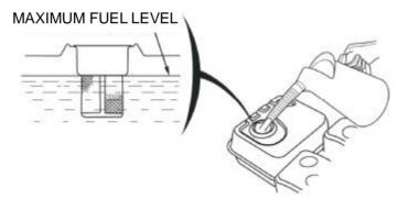
Refuel in a well-ventilated area before starting the engine. If the engine has been running, allow it to cool. Refuel carefully to avoid spilling fuel. Do not fill above the fuel strainer shoulder. After refueling, tighten the fuel tank cap securely.
