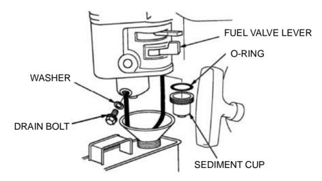
3. After all the fuel has drain into the container, reinstall the drain bolt and sediment cup.
