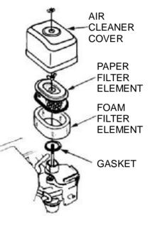
Paper air filter element: Tap the filter element several times on a hard surface to remove dirt, or blow compressed air [not exceeding 30 psi (207 kPa)] through the filter element from the inside. Never try to brush off dirt; brushing will force dirt into the fibers.
