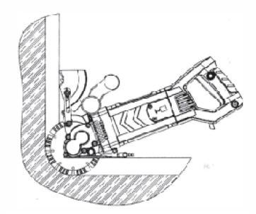
When the cover is turned over, it is used for cutting (slotting) wall corner.
