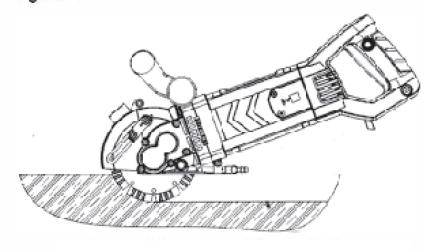
The state of a cover when the cover is closed.
