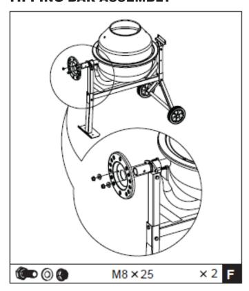
**1.** Slide the locking plate over the large diameter shaft at the leg end of the frame with the rim facing inwards as shown. Secure with two 8X25 bolts, each with a flat washer and a lock nut.
