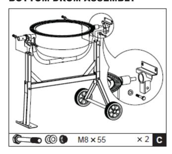
1. Slide the bracket onto the drive shaft sleeve.
