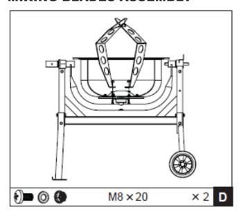
**4.** Mount the mixing blades inside the bottom drum loosely as shown - Two holes are provided at the base of the drum into which a M8X20 cross headed screw may be inserted from the outside. A leather washer and a lock nut should be threaded on loosely on the inside. The leather washer should be placed under the blade down against the drum.
