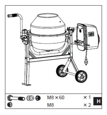
**3.** Lining up the keyways, slide the transmission case over the pinion shaft. Screw two lock nuts to the threaded stub on the transmission case. Secure the lower mount bracket to the frame with one M8X60 bolt, two flat washers and a lock nut.
