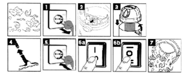
Unplug before change filter (Figure 1), then take out the bag and empty the dust or replace the bag. Slip the dust bag onto the socket(figure 2) for dry. vacuum-cleaning. Insert the plug and turn on the switch, then appliance starts to work (Figure 5 & 6a or 6b)
