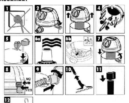
Figure 6a:Use the supplied foamed plastic filter for wet vacuumcleaning
