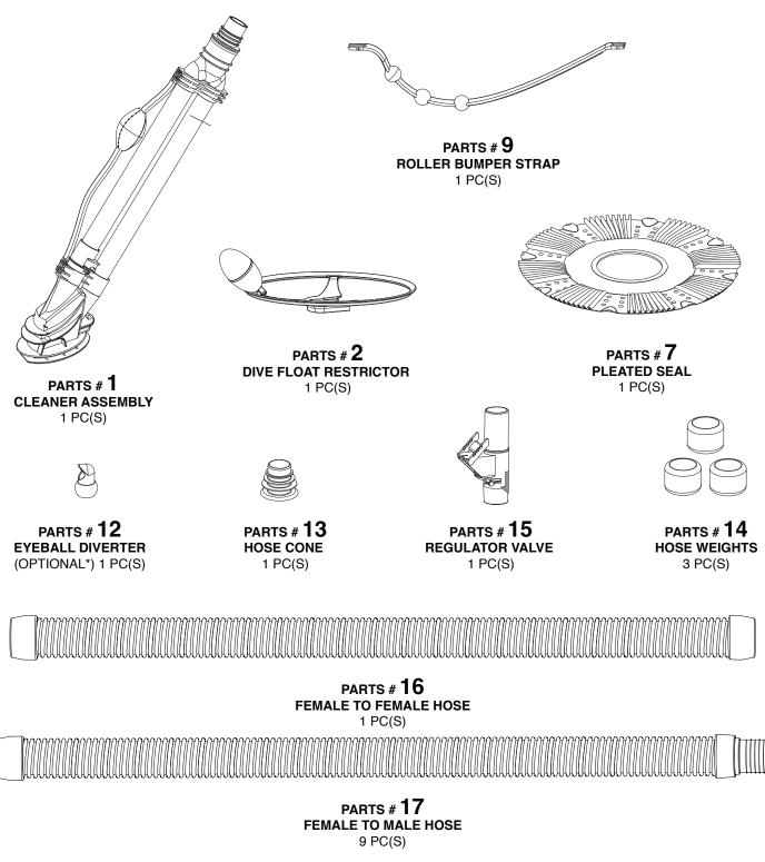
\*If the machine isn't covering the entire pool or is missing areas, adjust the eyeball diverter on the pool's return line.Rotate the diverter to face different directions to improve water flow and cleaner circulation. This may not be necessary for newer pools.
