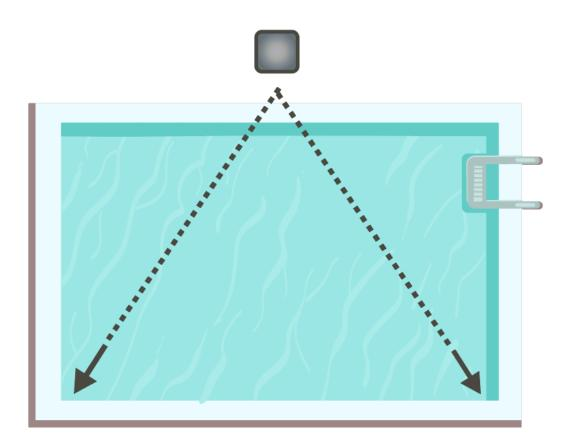
To ensure the best coverage of your pool, the power box should be placed at the middle point of the pool at least 12 feet from the pool's edge. Be sure to keep excess cord out of the pool.
