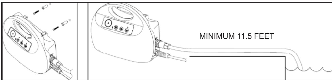
3. Put the Pool Cleaner into the pool. Release the Pool Cleaner and let it sink to the floor of the pool. Make sure that the floating cable is free of any obstructions.
