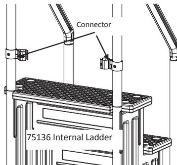
12. Fix the assembly to the top tread of the A Frame 75136, fix the connector by
