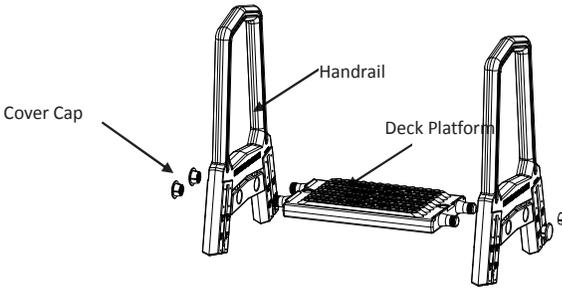
7. Attach handrails by pushing them down over the holders.
