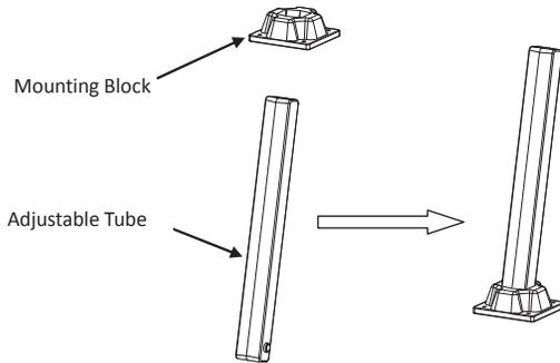
10. Fix the adjustable tube sets to the deck platform handrail with 10x1-1/4#
