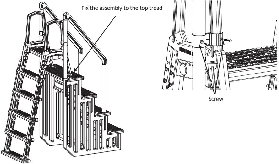
13. Fix the mounting block to the top tread by #10x1-1/4 screws
