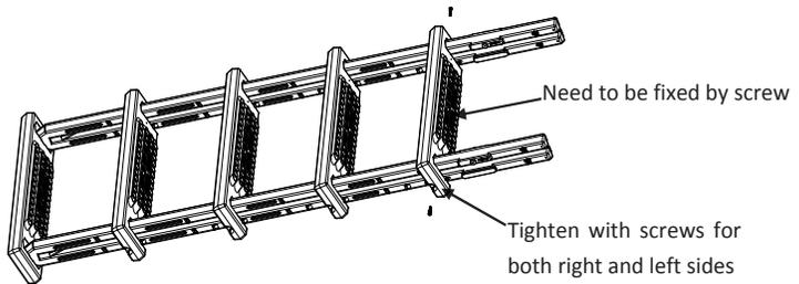
4. Fix the left and right fixing strips with bolt & gasket (M6), and nut M6\*85. Do not over-tighten
