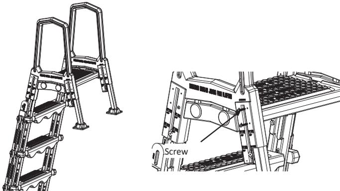
11. Put the connector to the handrails of the 75136 internal ladder
