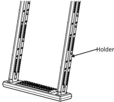
3. Install four treads to the holder, see the picture as below. Fix the top tread to the holder by #10 x 1-1/4 screws.
