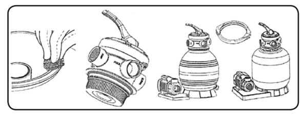
5. Connect the sand tank to the pump with hose and hose adapters.
