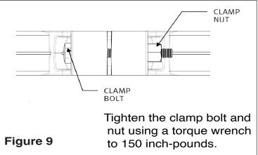
4. Do not rely on hand-tightening the clamp nut to the clamp bolt. Use a 3/4" socket on a torque wrench to tighten the clamp nut to the clamp bolt, applying 150 inch-lbs of torque (see Fig. 9).
