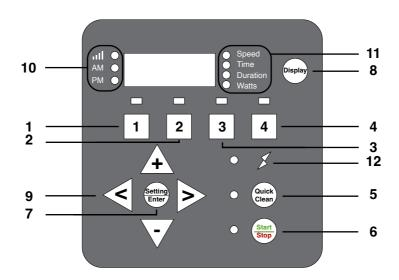
1 SPEED 1 Press to activate Speed 1 (2850 RPM).
