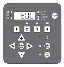
7. Set the duration using the + and - buttons, and adjust the cursor with < and >.
