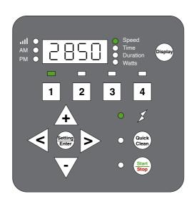
Adjust the Speed 1 RPM using the + and - buttons, and move the cursor with the < and > buttons.
