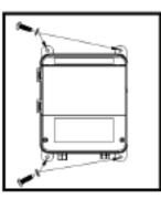
Fix the controller box on the wall and put gaskets on the screwws. Fasten the screws into the holes
