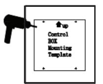
Secure mounting template to desired mounting location and drill mounting holes
