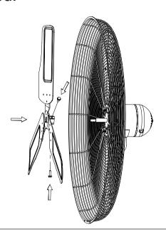
12. Secure the assembly of front guard and rear guard by tightening a screw and nut on the bottom and position of them.
