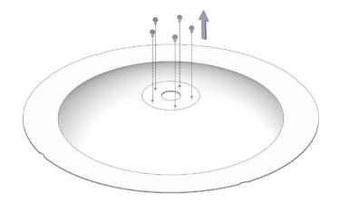
2. Attach support post to base by tightening with the five screws from Step 1.
