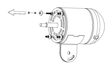
8. Set rear guard in proper position and fix it to fan head by securing back the hexagonal nuts, spring and washers and big washers from Step
