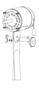
7. Remove four sets of hexagonal nuts, spring washers and big washers from fan head. Save them for Step 8.
