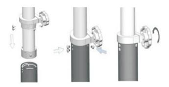
6. Mount fan head onto extension pipe by tightening back the hexagonal bolt, bolt sheath and washer.
