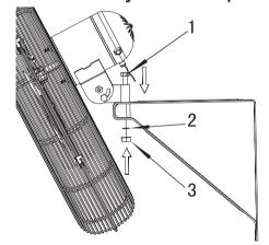
4. Loose Washer Nut M8 for adjusting the desired tilt angle of Fan Head, and fix it again.
