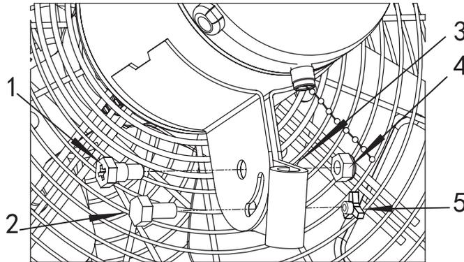
3. Assemble the Upper Bracket with the wall bracket by screws as follow:
