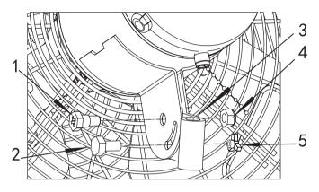
3. Assemble the Upper Bracket with the wall bracket by screws as follow: Firstly, insert No. 1 Screw M12×100 through the Upper Bracket Secondly, connect the Lower Bracket with Upper Bracket by No. 1 Screw Finally, fasten two bracket by No. 2 Spring washer and Hexangular Nut M12
