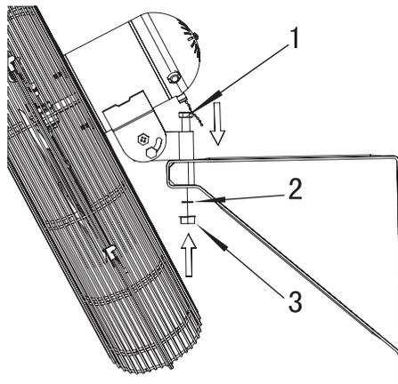
4. Loose Washer Nut M8 for adjusting the desired tilt angle of Fan Head, and fix it again.
