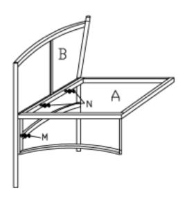
**STEP 1:**Connect left frame B and seat frame **A** with bolt **N** and secure wit the allen key.
