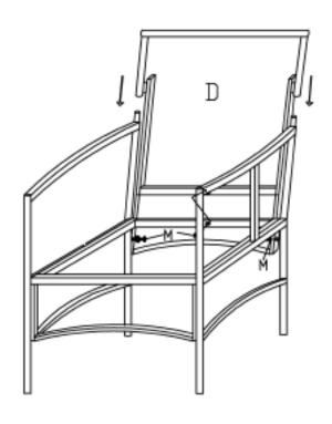
**STEP 3:**Connect the parts from step 2 and back frame **D** with bolt **N** with an allen key.
