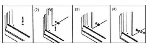
**Step 2.** Insert the cam bolts (21) into the left vertical front panel (3). Then insert the cam bolts (21) into the left side panel (2), tighten by rotating the cam locks (22) clockwise with a Phillips screwdriver.
