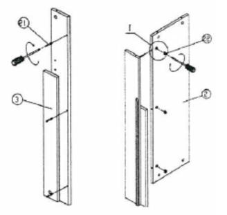
**Step 4.** Attach assembled unit on Step 2 and assemble unit on step 3 to the base on step 1 using cam bolts (21) into the corresponding holes onto base (1). Tighten by rotating cam locks.
