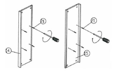
**Step 16.** Attach assembled unit on step 10 to fixed panel (16) by cam bolts (21) into corresponding holes into the fixed panel. Tighten by rotating cam locks clockwise with screwdriver.
