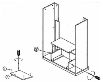
**Step 9.** Screw cam bolts (21) into holes on top panel (8). Attach top panel to assemble unit on step 8 by cam bolts (21) into corresponding holes until top panel (8) and assemble. Tight by rotating cam locks clockwise with screwdriver.
