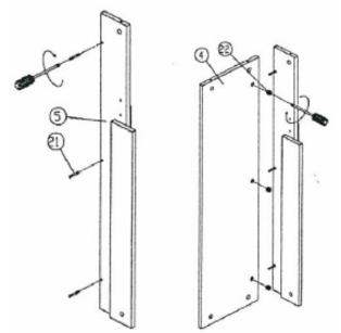
**Step 5.** Tighten lower front (9) panel to the unit on step 4 by screw (23)
