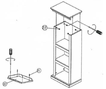
**Step 15.** Insert the cam bolts (21) to the left side panel (14) and the right side panel (15). Tighten by rotating cam locks with screwdriver.
