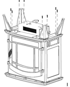
Insert the leg buckles into the holes located on the base of the stove. Fasten the legs using the screws (1 screw per leg) and tighten with a Phillips head screwdriver, as followed picture.
