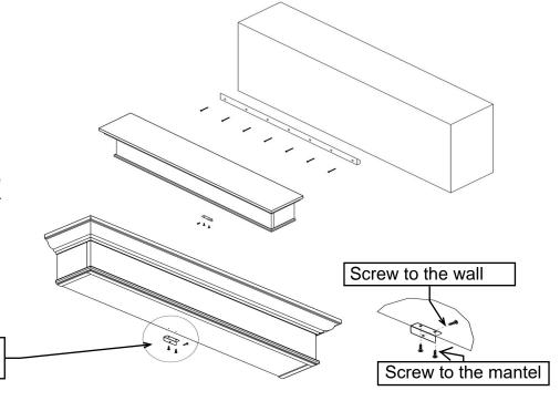
Bottom bracket must be installed to ensure safety.
