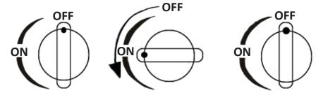
**3.** When the knob is turned to the 90 degree position, the firepower is the maximum. You can continue to adjust the firepower counterclockwise or clockwise.
