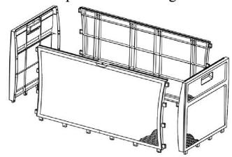
Step 2: Fix the frame of front, back and side panels with the bottom.
