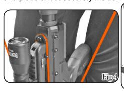
**6.** Pull both t-handles simultaneously, drawing the crossbow string back under the bolt retention spring into the string opening of the trigger mechanism.
