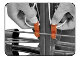
**7.** Place the arrow/bolt so that the cocking vane is down in the flight groove.
