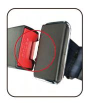
Press red button to unlock seat belt and belt will retract to right side of seat
